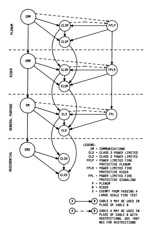
Fig. 2—Permitted Interchanges of Listed Cables
