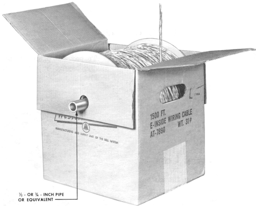
Fig. 4 — Carton Used as Reel Support
