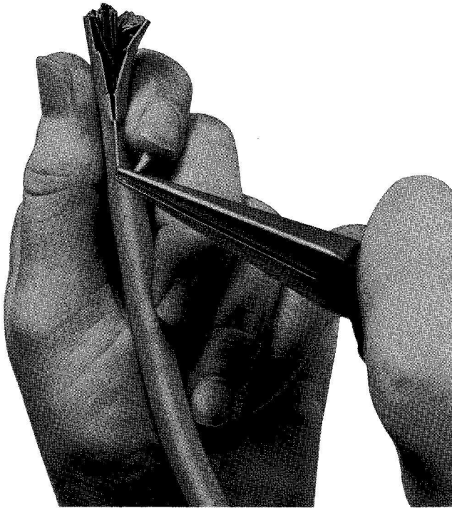
Fig. 7 — Stripping IW Cable (with Jacket-Splitting Cord)
