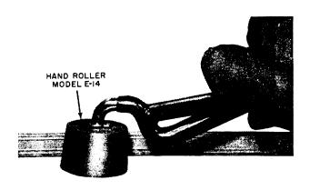
Fig. 3—Applying Roller to Wire Run
