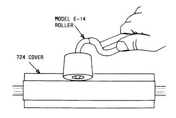
Fig. 14—Installing No. 724 Station Wire Cover
