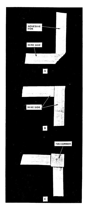
Fig. 4-90° Turn in B Station Wire
