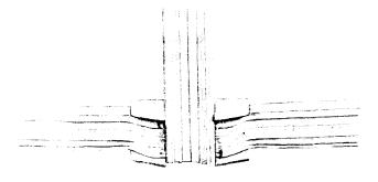
Fig. 9-Wire Tap Using No. 718 Tap
