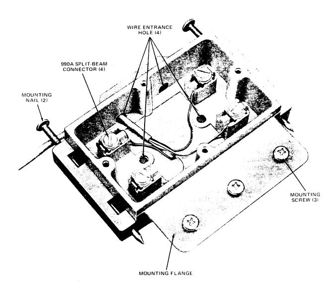
Fig. 1—800C Station Wire Box (Without Temporary Cover)
