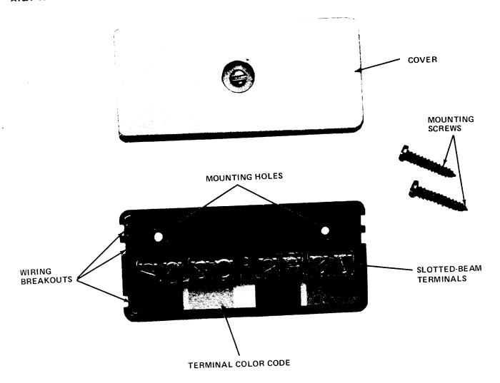
Fig. 9—742B Connecting Block
