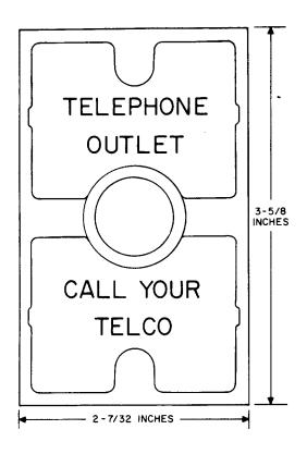
Fig. 2—Temporary Cover (800C Station Wire Box)
