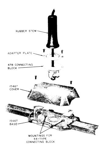
Fig. 4-1546T Telephone Outlet
