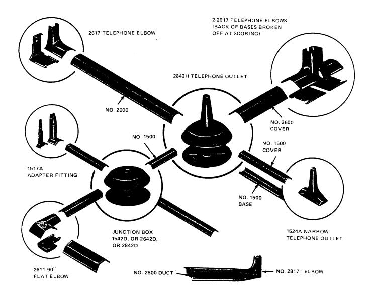
Fig. 1—Wirehold Metal Overfloor Duct
