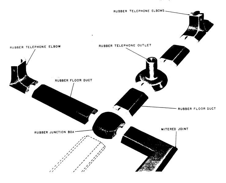
Fig. 3—B Rubber Overfloor Duct
