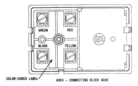
Fig. 17—725S-S Connecting Block
