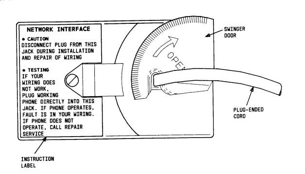
Fig. 13—625TD-Type Connecting Block
