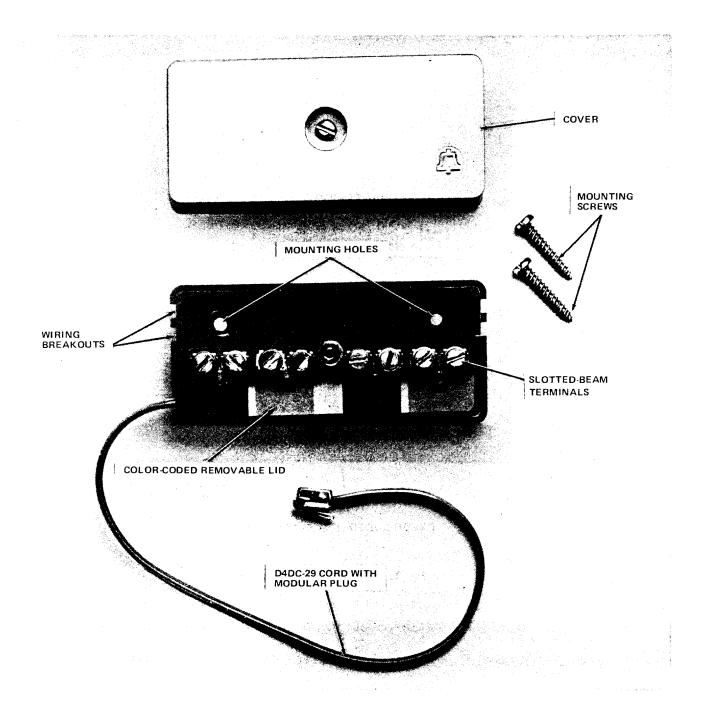
Fig. 14-742A-S Connecting Block
