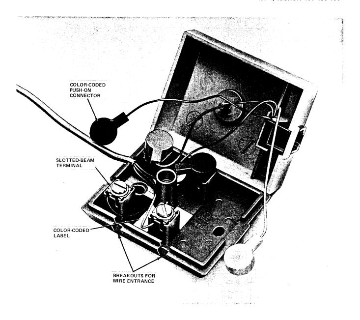
Fig. 16-725A-S Connecting Block
