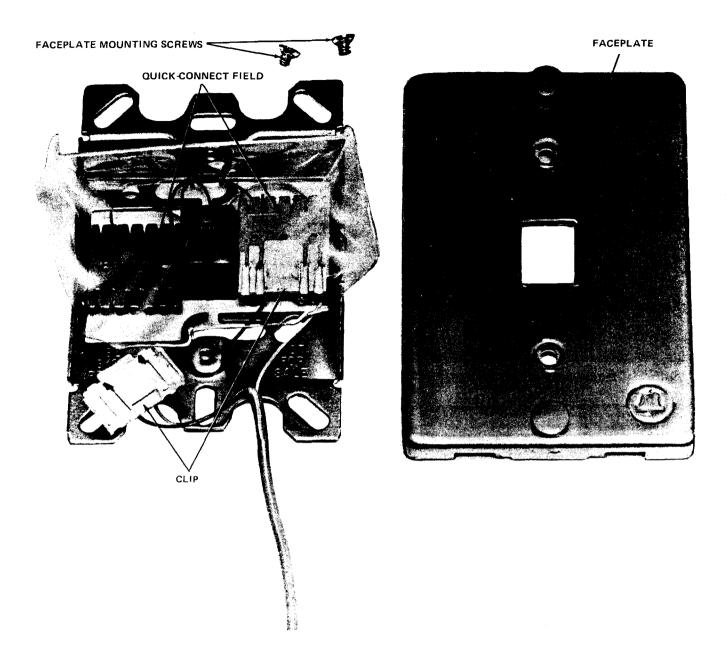
Fig. 4—630B-S Connecting Block
