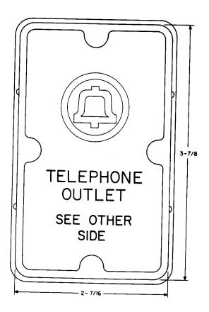
Fig. 2—Protective Cover for 800A Station Wire Box
