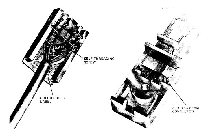
Fig. 1—700A-S Plug With Conductors Terminated
