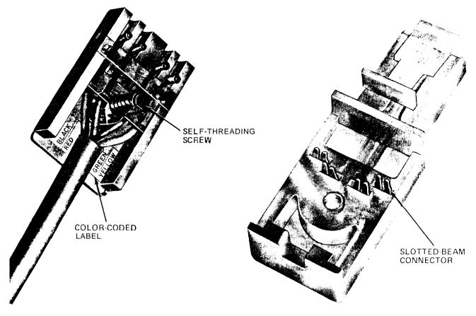
Fig. 27.1 -700A4 Plug With Conductors Terminated
