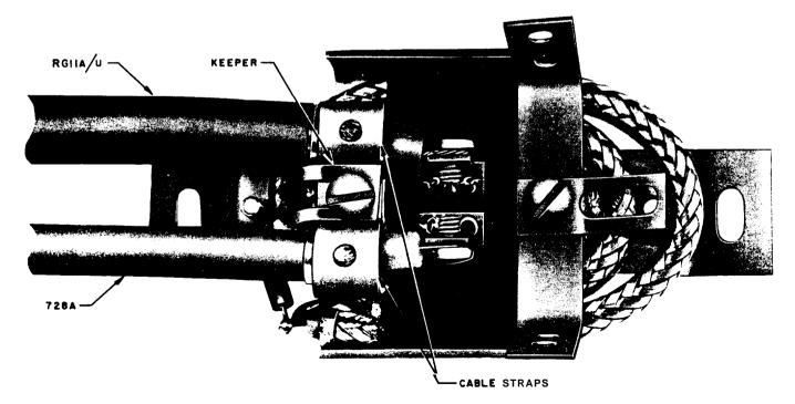
Fig. 4 - SKL 964-16U Jack with Cable Attached
