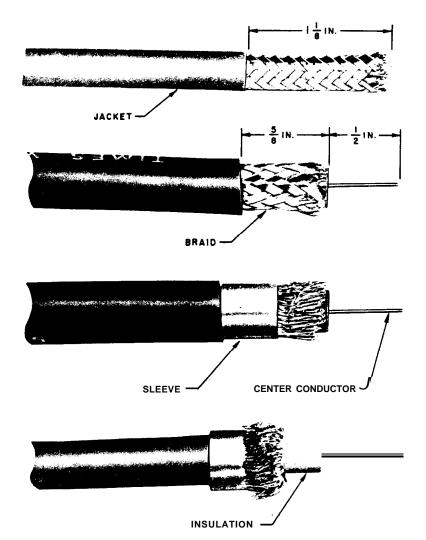
Fig. 2 - Stripping 728A and RG11A/U Coaxial Cable
