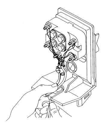
Fig. 5—Placing Wires Through Horseshoe Grommet
