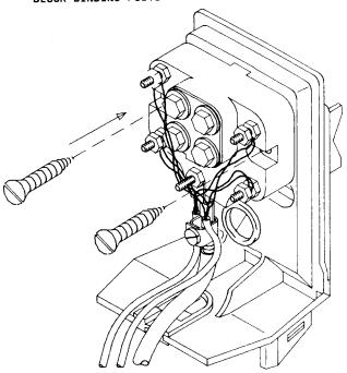
Fig. 4—Mounting Protector Block to Base
