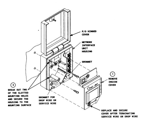
Fig. 2-Mounting 100-Type NIU
