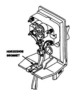
Figure 18. Securing Wires in Grommet
