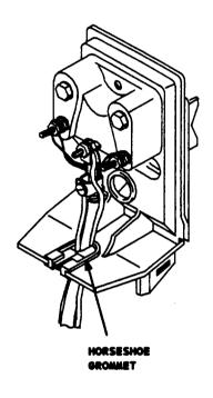
Figure 15. Securing Wires in Grommet
