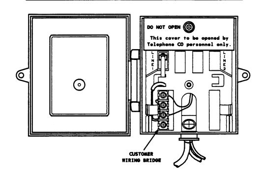
Figure 11. Attaching Customer Wiring to Customer Bridge
