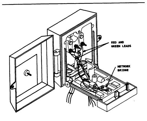
Figure 10. Attaching Leads from Network Bridge to Protector
