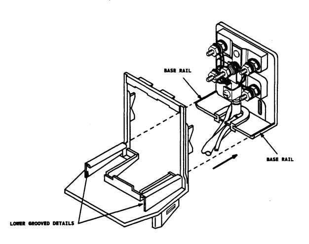
Figure 20. Sliding Adapter Along Base Rails
