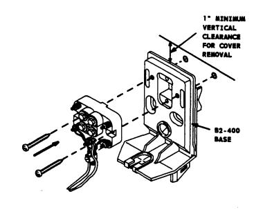
Figure 17. Mounting Protector/Base Assembly
