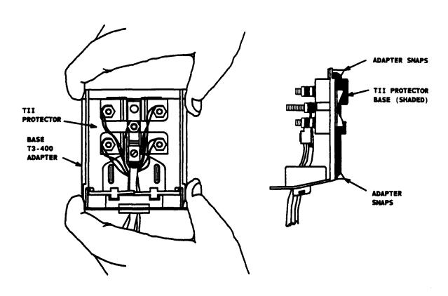
Figure 21. Snapping Adapter onto Base
