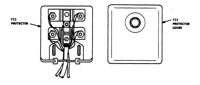
Figure 19. Removing Cover of TII Protector
