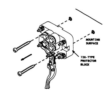
Figure 16. Removing Cover of TII Protector
