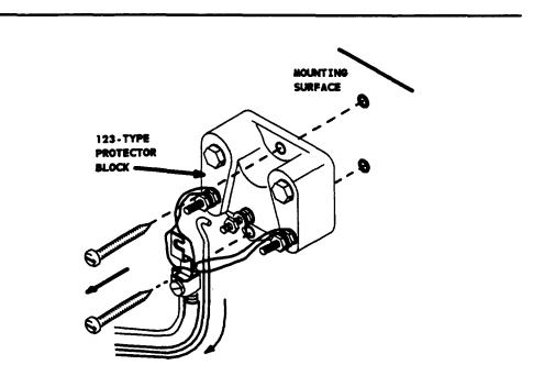
Figure 13. Removing Protector Block from Mounting Surface
