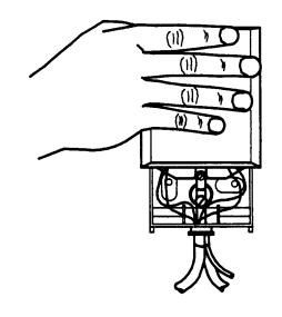
Figure 7. Removing Cover of B Customer Service Closure
