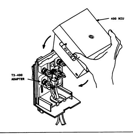
Figure 22. Installing 400 NIU onto Adapter
