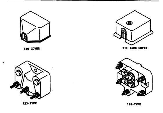
Figure 12. Identification of Protector Cover and Protector Type
