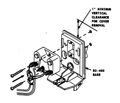
Figure 14. Mounting Protector Block and Base to Mounting Surface
