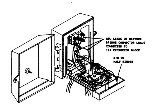
Figure 9. 401 NIU - Wiring MTU to Protector Unit
