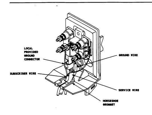
Figure 6. 401 NIU — Completing the Protector Wiring
