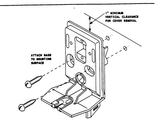
Figure 5. 401 NIU - Mounting Base onto Wall
