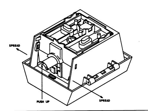
Figure 4. 401 NIU - Disassembly
