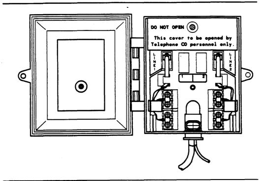
Figure 7. 401 NIU — Installing Network Interface Unit onto Base
