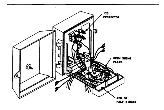
Figure 8. 401 NIU With Swing Plate Open
