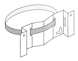
Fig. 6—Mounting the SNI-2125 to a pole.
