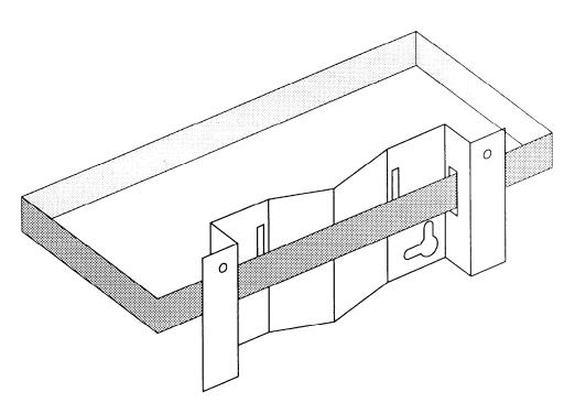
Fig. 5—Mounting the SNI-2125 to an I-beam.
