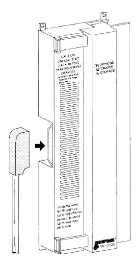
Fig. 3—Connecting 25-pair cable to the SNI-2125
