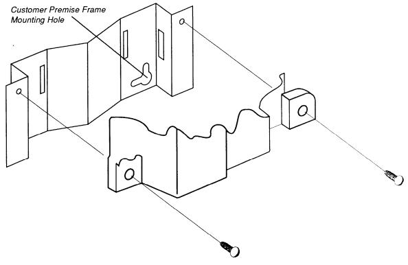
Fig. 4—Mounting the SNI-2125 to the Auxiliary Mount Brackets.
