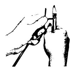
Fig. 7—Crushing Insulation
