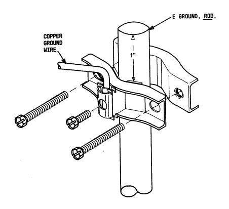
Fig. 2—Ground Wire Attachment to E Ground Rod
