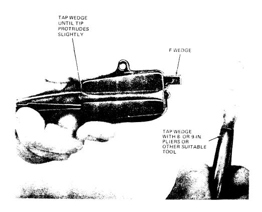
**♦Fig. 4—Securing Drop Wire**
