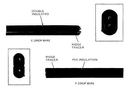
Fig. 7—F Drop Wire and C Drop Wire
