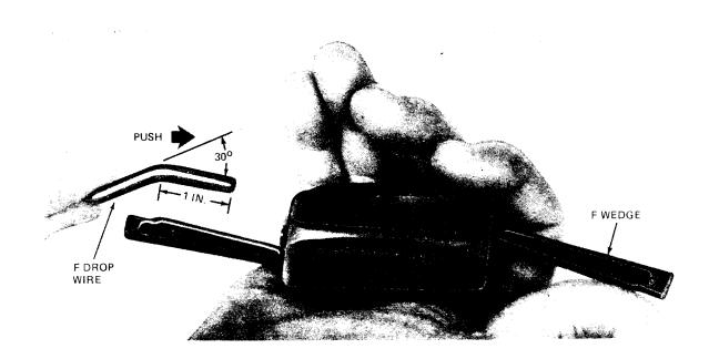
Fig. 3—Inserting F Drop Wire
