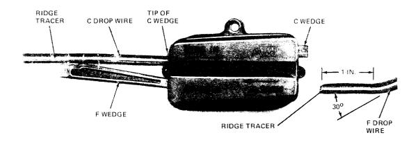
Fig. 10—Splicing C Drop Wire to F Drop Wire
