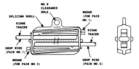
Fig. 2—B Drop Wire Splice—Cutaway
