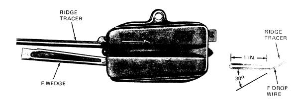
Fig. 5—Aligning Ridge Tracers
