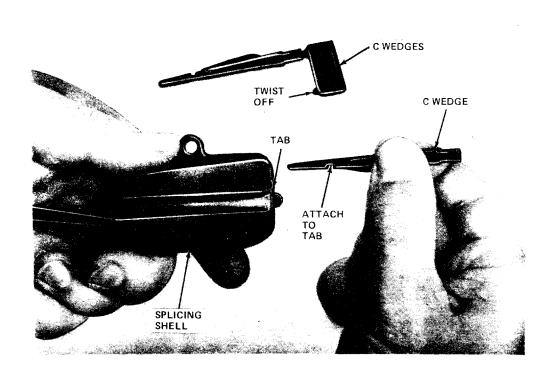
♦Fig. 8—Installing C Wedge
