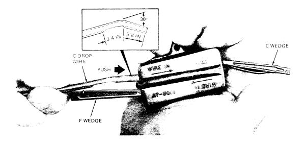
**♦**Fig. 9—Inserting C Drop Wire
