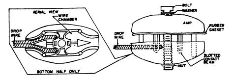
Fig. 3 - Drop Wire Insertion
