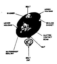
Fig. 1 - AMP\* Mini Drop Wire Splice
