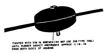
Fig. 4 - Completed Splice
