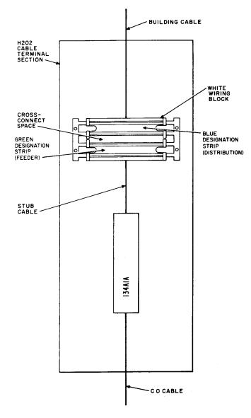
Fig. 8—Entrance Cable and Building Cable Terminating on One Wiring Block
