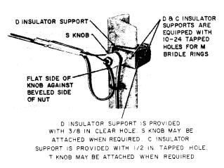
Fig. 14—₱First Attachment—D or C Insulator Support●
