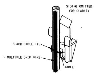
Fig. 30 — ♦B Siding Clip With F Multiple Drop Wire €
