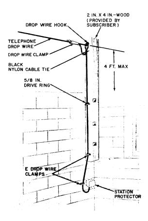
Fig. 21—Drop Wire Attached to 2- x 4-Inch Wood Beam
