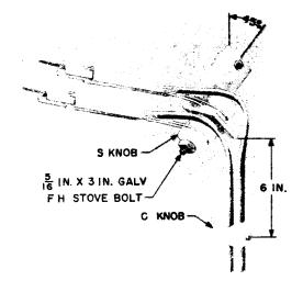
Fig. 10—First Attachment—House Bracket (Vertical Run, Double Wire) With S Knob
