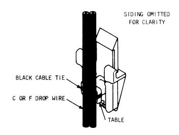
Fig. 29 — ♦B Siding Clip With Cord Drop Wire¶
