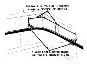
Fig. 24—♦Spacing Attachments at Inside Corner of Building♦
