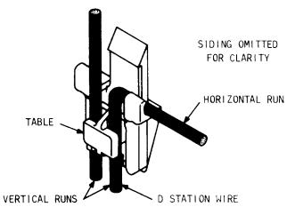
Fig. 28 — ♦B Siding Clip With Two D Station Wires ♦
