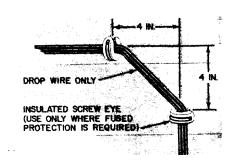
Fig. 25—♦Spacing Insulated Screw Eye When Changing Direction of Wire Run€
