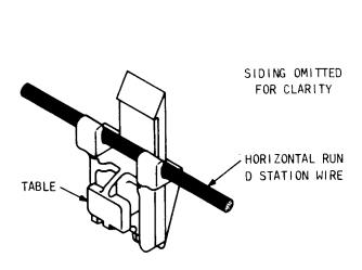
Fig. 27 — ♦B Siding Clip With D Station Wire¶
