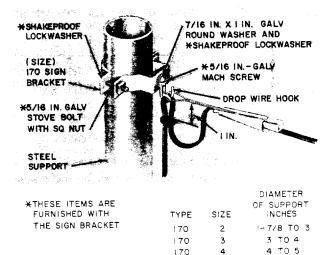
Fig. 15—₱First Attachment—Sign Bracket, 170-Type¶
