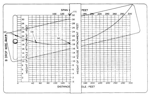
NOTE RULE APPLIES ONLY WHEN DROP WIRE IS TO BE STRUNG TO MINIMUM DROP WIRE SAGS IN 462 - 400 - 200.
