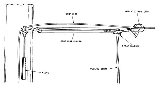
Fig. 3 - Tensioning Drop Wire
