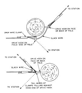
Fig. 7 - Distributing Wires From Pole Without Terminal
