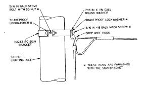
Fig. 9 - Attachment to Type 170 Sign Bracket
