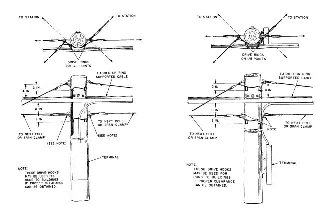
Fig. 2 - TERMINAL MOUNTED ON CABLE SIDE OF POLE Fig. 3 - TERMINAL MOUNTED ON FACE OR BACK OF POLE
