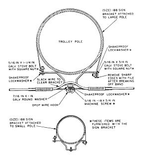
Fig. 10 - Attachment to Type 188 Sign Bracket
