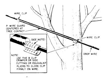
Fig. 4—Protection For Wire At Tree Contact Larger
