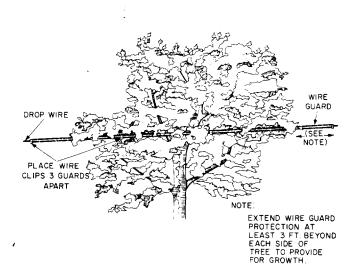
Fig. 6-Protection For Wire Through Tree
