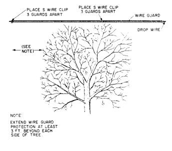
Fig. 5-Protection For Wire Over Tree
