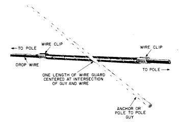
Fig. 7—Protection For Wire At Guy in Span
