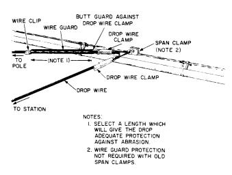
Fig. 8—Protecting Wire From Abrasion At Span Clamp on Strand For Ring Supported Cable
