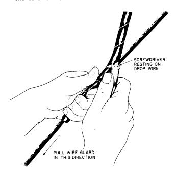
Fig. 3—Placing P Wire Guard Screwdriver Method
