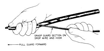
Fig. 2-Placing P Wire Guard Hook Method
