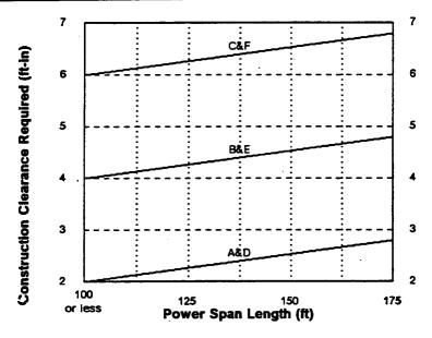
NOTE: Maintenance clearances for span lengths of 101 to 175 feet are to be the same as that specified in placing the drop wire for span lengths of 100 feet or less.
