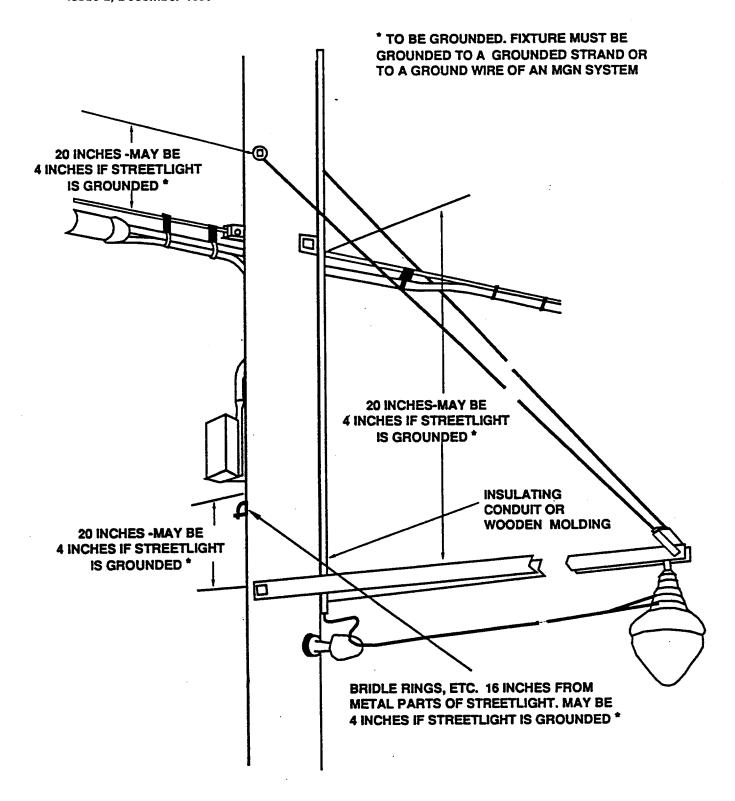
Figure 3-2. Clearance of Drivehooks, Bridlewire Rings, or Brackets from Streetlight Fixture
