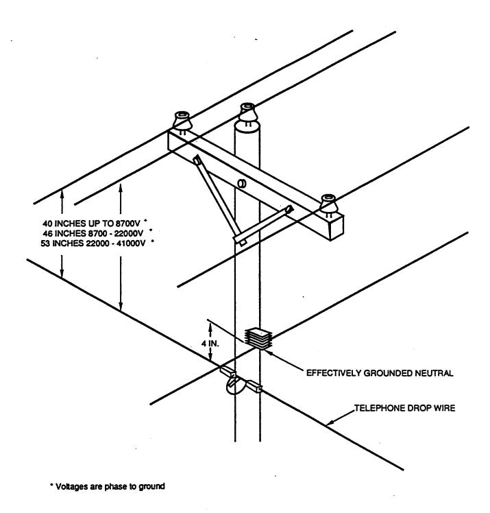
Figure 3-6. Multiple Drop Wire Clearance on Common Crossing Pole
