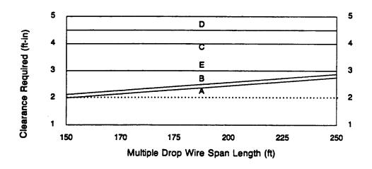
Figure 3-8. Multiple Drop Wire Placing Clearances - Medium Loading Area - Above, Below, or Alongside Electrical Facilities - with Normal and Minimum Sag.
