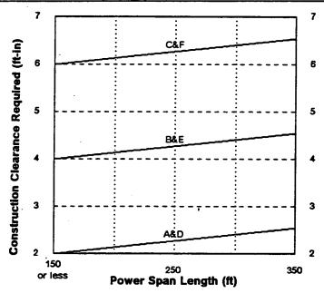
NOTE: Maintenance clearances for span lengths up to 350 feet are to be the same as that specified in placing the drop wire for span lengths of 150 feet or less.
