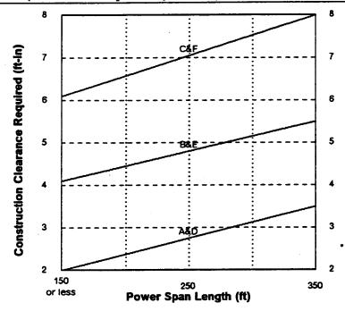
NOTE: Maintenance clearances for span lengths up to 250 feet are to be the same as that specified in placing the drop wire for span lengths of 150 feet or less.
