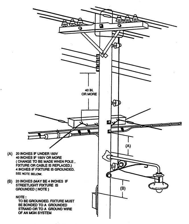
Figure 3-4. Clearance of Cable and Pole-Mounted Terminal from Streetlight Fixture Mounted Below Cable
