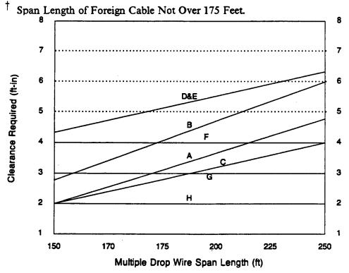
Figure 3-9. Multiple Drop Wire Placing Clearances - Heavy Loading Area - Above, Below, or Alongside Electrical Facilities - with Normal and Minimum Sag.
