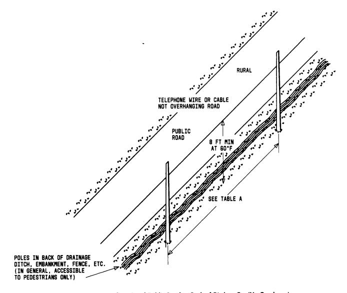
Fig. 6—Running Along Rural Public Roads—Back of Ditches, Etc (No Overhang)
