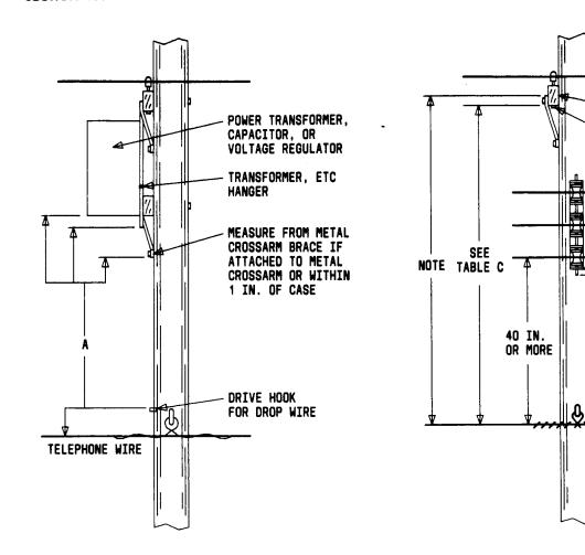
Fig. 13—Vertical Clearance From Power Transformer, Crossarm Braces, Etc
