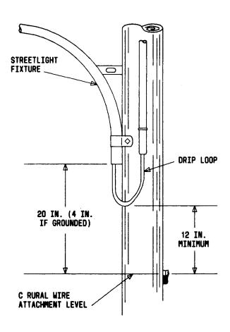
Fig. 15—Clearance From Streetlight Fixture Drip Loop
