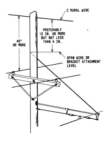
Fig. 17—Clearance Between C Rural Wire and Trolly Wire and Attachments
