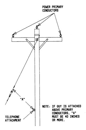
Fig. 18—Clearance Between Power Guys and Telephone
