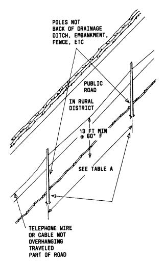
Fig. 7—Running Along, But Not Overhanging, Public Roads (Not Back of Obstruction)
