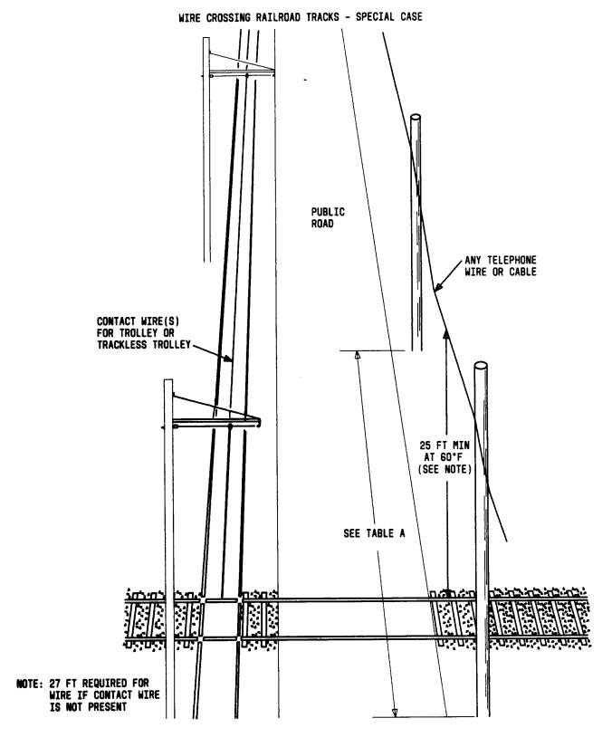
Fig. 5—Wire Crossing Railroad Tracks—Special Case
