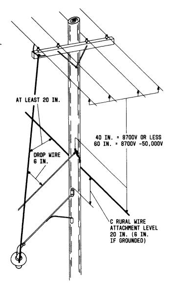
Fig. 16—Clearance of Streetlight Vertical Feed Wire From C Rural Wire
