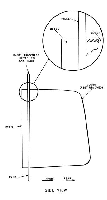
Fig. 7—106-Type Loudspeaker Set, Panel Mounted
