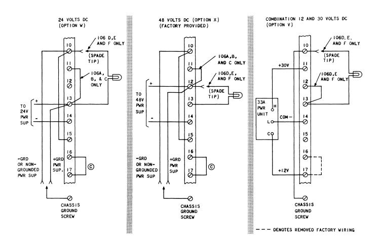
Fig. 9—Connections for 106-Type Loudspeaker Set—Power Supply Options
