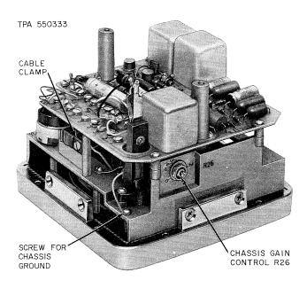
Fig. 5-106D, E, or F Loudspeaker Set, Cover Removed
