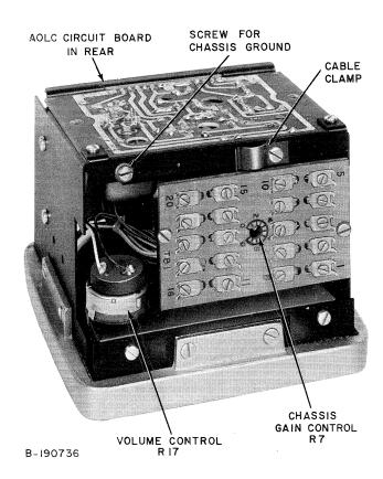
Fig. 3—106C (MD) Loudspeaker Set, Cover Removed
