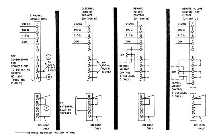
Fig. 8—Connections for 106-Type Loudspeaker Set—Feature Options
