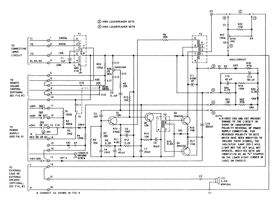
Fig. 13—Schematic—106D and E Loudspeaker Sets
