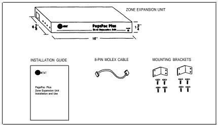
Figure 1. Zone Expansion Unit Components
