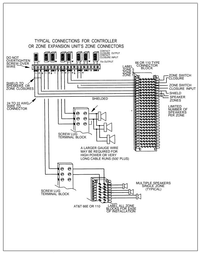
Figure 8. Zone Wiring Using Connector Blocks
