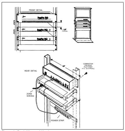
Figure 3. Rack Mounted Hardware
