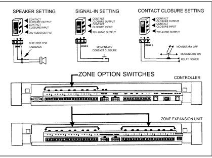
Figure 6. Setting Zone Option Switches on Controller and Zone Expansion Units
