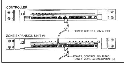
Figure 4. 8-pin Molex Connector from Controller to Zone Expansion Unit(s)
