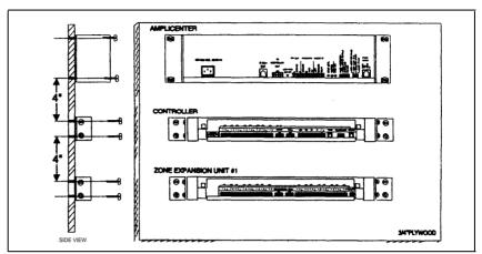
Figure 2. Wall Mounted Hardware
