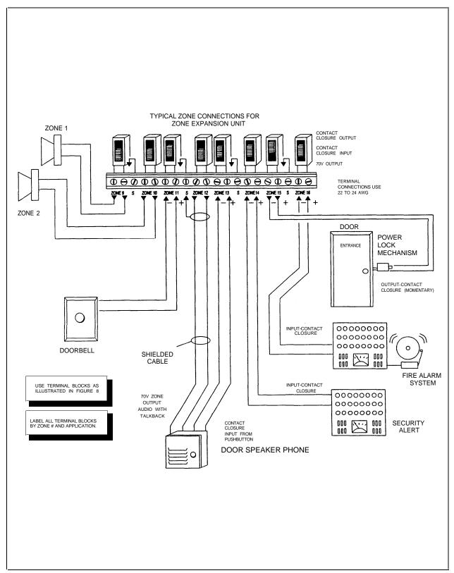
Figure 9. Contact Closure Zone Wiring to Zone Expansion Units and Controller
