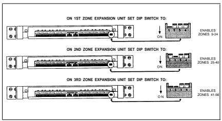
Figure 5. Setting Zone Expansion Unit DIP Switches
