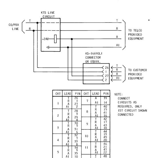
Fig. 3—Connections for USOC RJ22X—Multiple Bridged Tip and Ring Ahead of Line Circuit With "A" Lead Control
