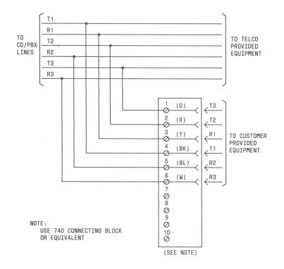
Fig. 2-Connections for USOC RJ25C
