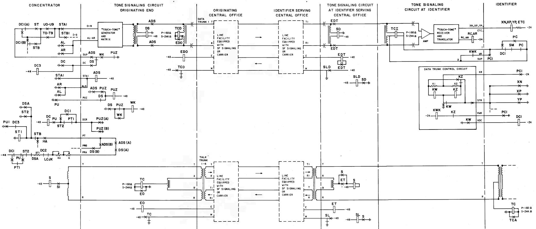
Fig. 1—Functional Schematic of Tone Signaling Circuit for Use With Line Concentrator-Identifier
