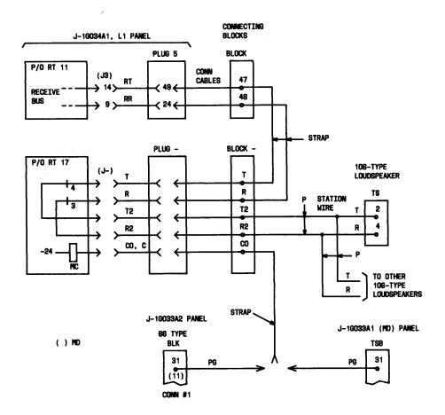
Fig. 27—PLoudspeaker Connections, Speaker Cut Off When Privacy is Initiated in a Privacy SS-4 System
