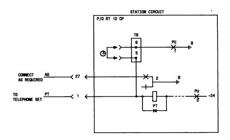
Fig. 30—AG Lead Ground, for Special Applications
