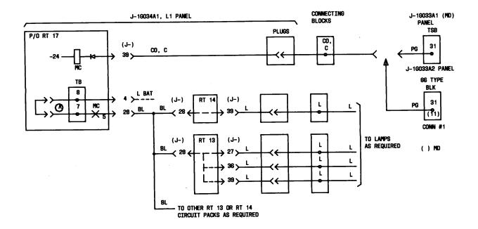
Fig. 19—Connections for A Option
