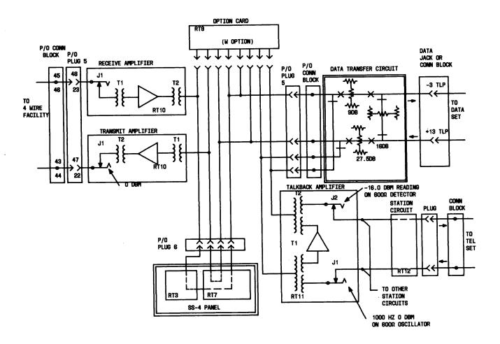
Fig. 32—▶Typical Transmission Diagram, SS-4 With Data Access
