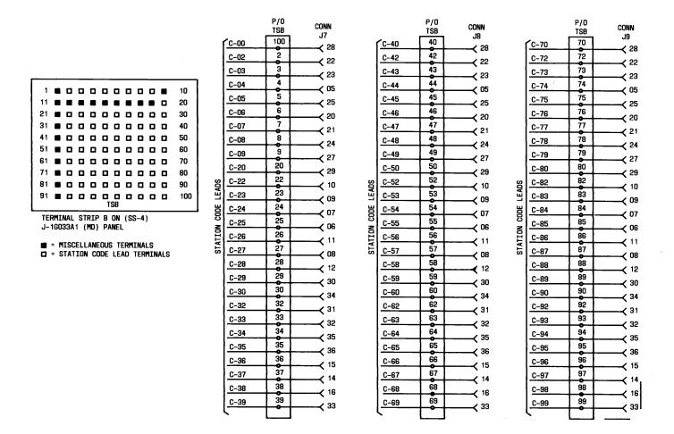
Fig. 13—Station Code Lead Terminals on J1G033A-1 (MD) SS-4 Panel
