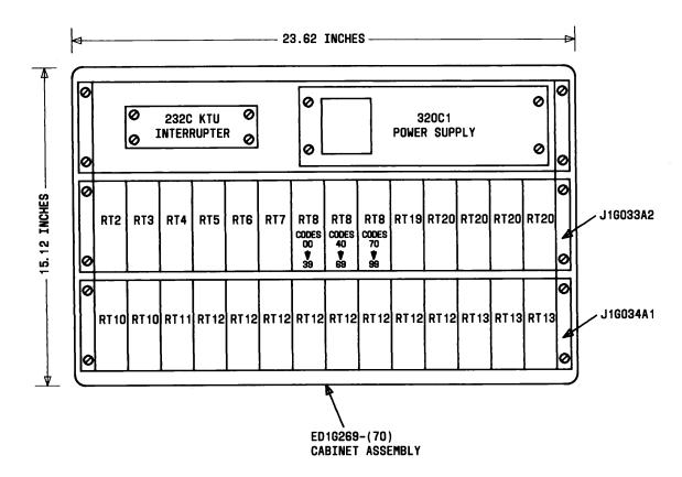
Fig. 5—₱J1G033B SS-4 Packaged System E/W Eight Station Circuits and TOUCH-TONE Dialing (Front View Cover Removed)◀
