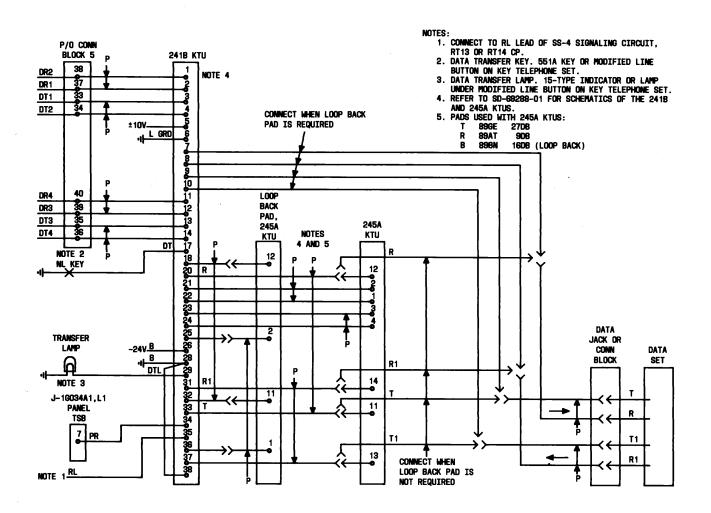
Fig. 25—Data Transfer Circuit
