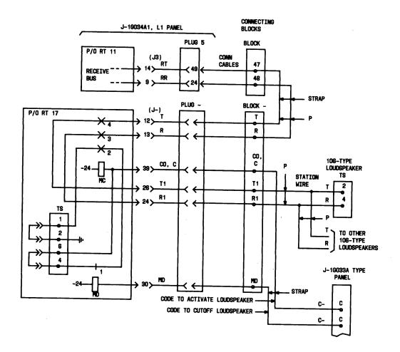
Fig. 28—Doudspeaker Connections, Speaker Activated and Cut Off by SS-4 Codes€
