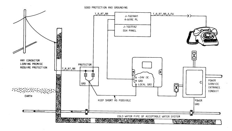
Fig. 33—System Grounding
