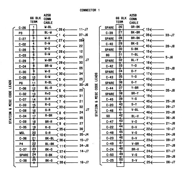
Fig. 14—♦Station and Miscellaneous Code Leads for J1G033A-2 Apparatus Option F (MD) SS-4 Panel (Sheet 1 of 2)♦
