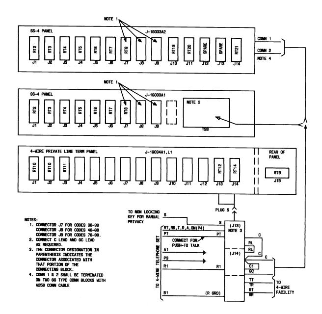
Fig. 11—PConnections for One 4-Wire Telephone Set (Sheet 2 of 2) €
