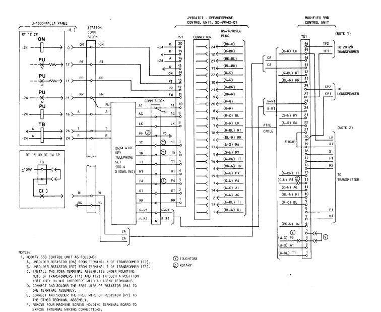
Fig. 23—3A Speakerphone Connections
