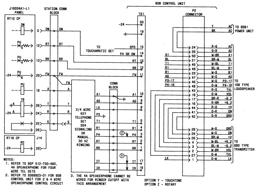
Fig. 24—♦4A Speakerphone Connections •
