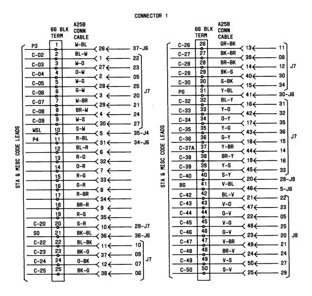
Fig. 15—♦Station and Miscellaneous Code Leads for J1G033A-2 Apparatus Option E (Issue 9B or Later) SS-4
