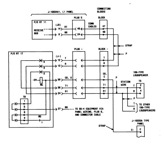
Fig. 29—Doudspeaker Connections, Speaker Activated by SS-4 Code, Automatic Cutoff
