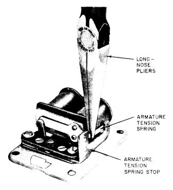
Fig. 17—♦Adjusting Armature Tension Spring, 7-Type
