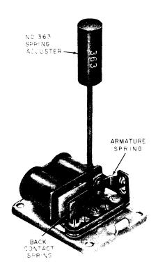
Fig. 18—♦Adjusting Armature Spring, 7-Type Buzzer♦
