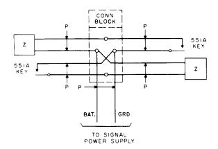
Fig. 22—Small Pushbutton and Buzzer System
