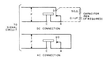
Fig. 23—AC and DC Connections
