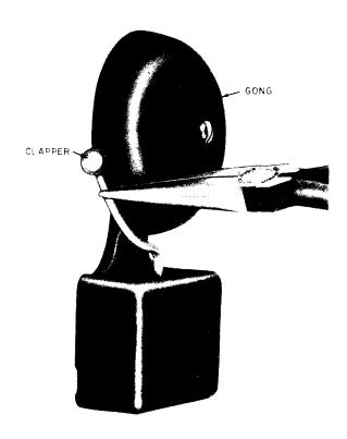
Fig. 19—♦Adjusting Clapper Movement, 7-Type Bell
