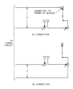
Fig. 24—KS-8108, KS-8109, and KS-8110 Type Buzzer Connections
