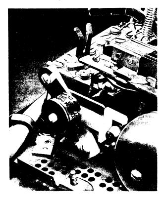
Fig. 10—KS-20419 Type Buzzer Mounted on Bracket of H1A Ringer
