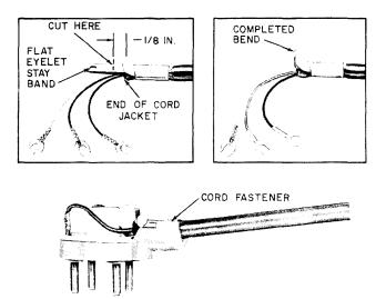
Fig. 2—Connecting Current Model D3BU or D4BP Cord To Early Model 505A Plug
