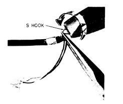
Fig. 4—Bending S Hook
