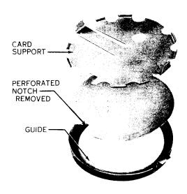
Fig. 2—Method of Placing Card in Holder
