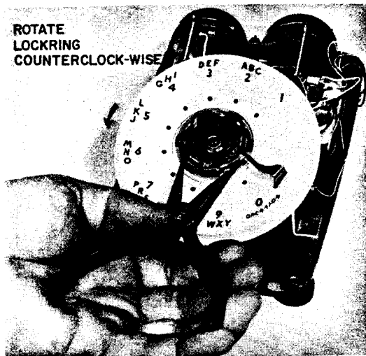
Fig. 9—Lockring Removal
