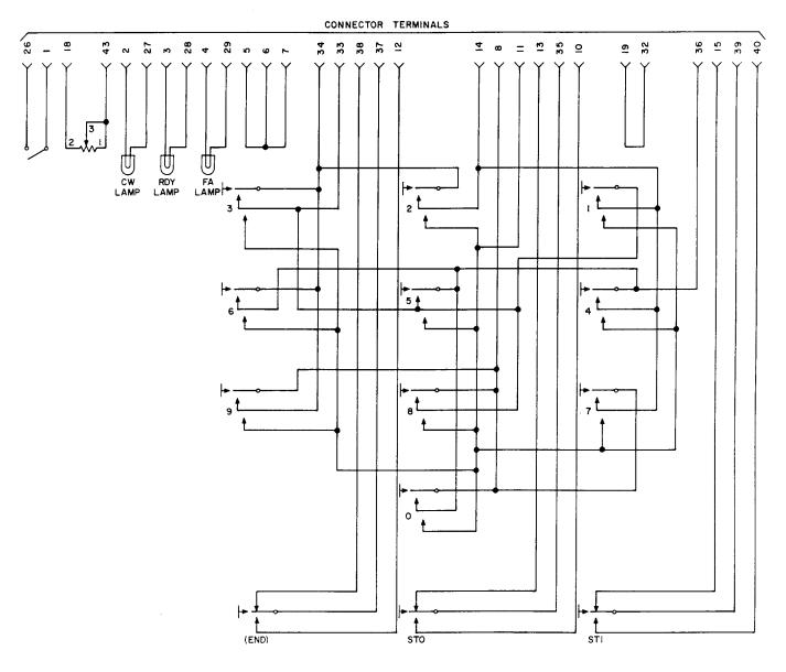
Fig. 6-21D Dial Schematic
