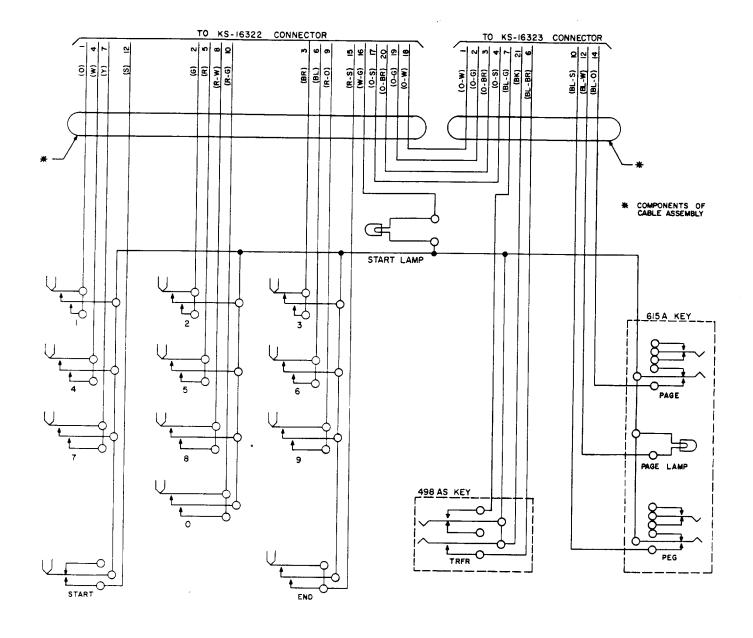
Fig. 5 – 23A Dial, Wiring Schematic
