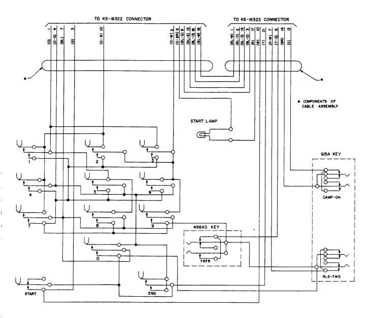
Fig. 6 – 23B Dial, Wiring Schematic
