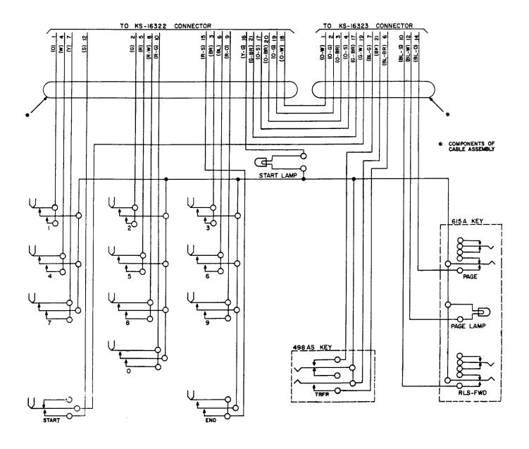
Fig. 7 — 23C Dial, Wiring Schematic
