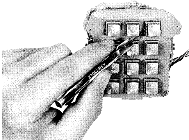
Fig. 8—Removing Special Service Button
