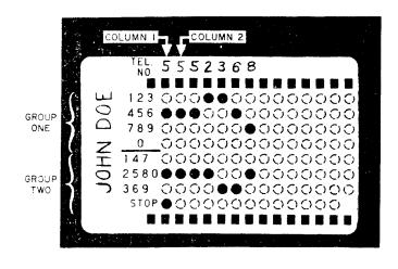
Fig. 5 — Card Coded for 7-Digit Telephone Number
