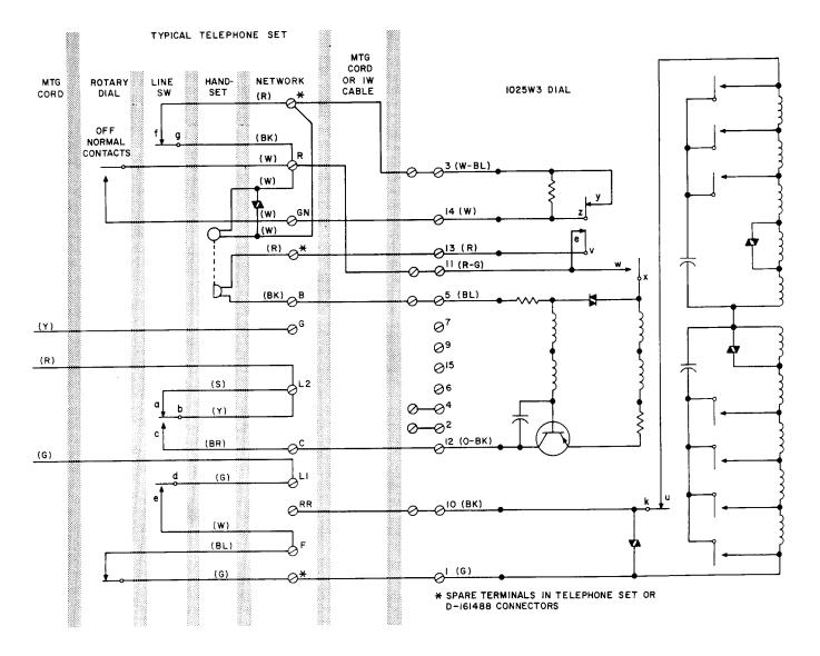
Fig. 4-1025W3 Dial, Typical Connections to Rotary Dial Telephone Set
