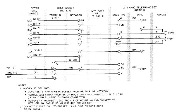
Fig. 6—1025W3 Dial, Connections to 211J Hand Telephone Set Using 685A Subscriber Set
