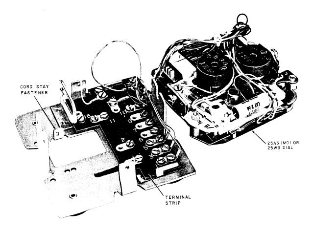
Fig. 2—1025-Type Dial, With Cover Removed
