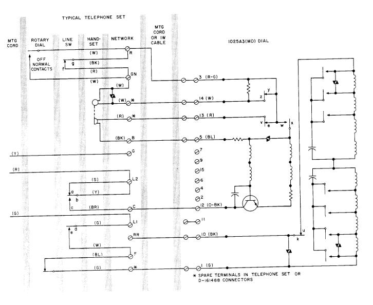
Fig. 3—1025A3 (MD) Dial, Typical Connections to Rotary Dial Telephone Set
