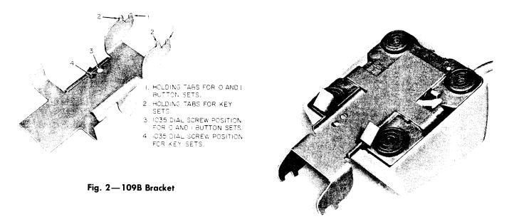
Fig. 3—1035C3A (MD) or 1035AF3A Dial Mounted on 109B Bracket
