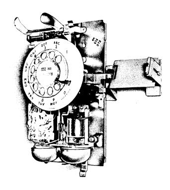
Fig. 8—D-180644 Kit of Parts Installed on Wall Telephone Set
