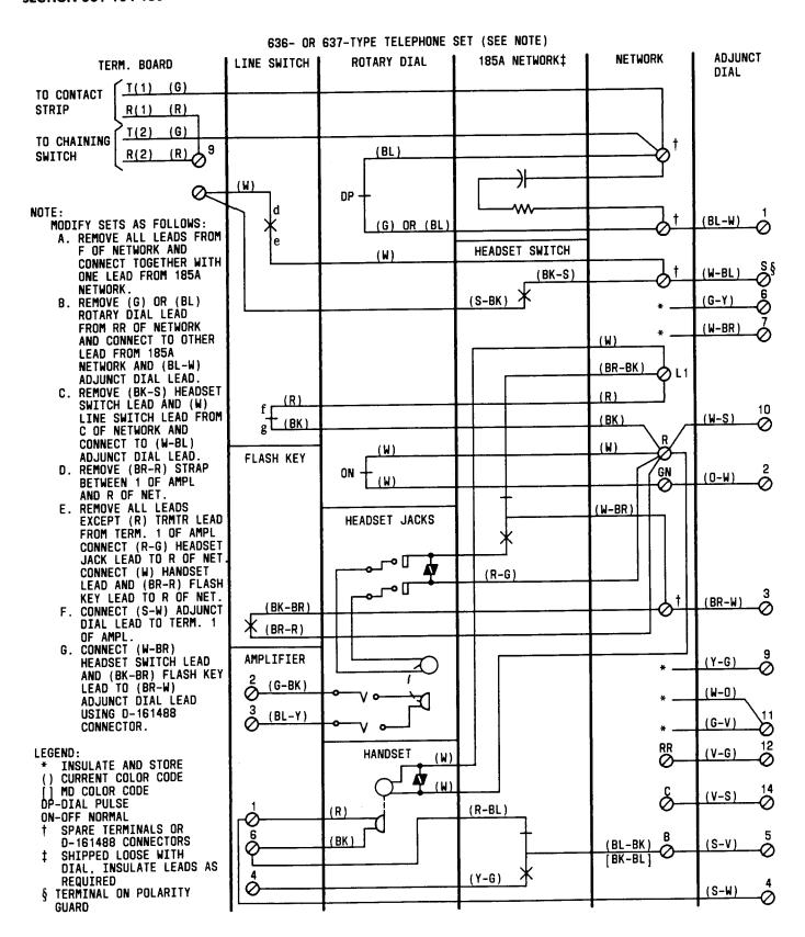
Fig. 22—1035C3A (MD) or 1035AF3A Dial, Connections to 636- or 637-Type Telephone Set
