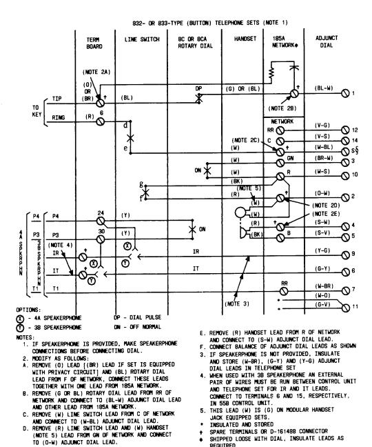
Fig. 27—1035C3A (MD) or 1035AF3A Dial, Connections to 832- or 833-Type Telephone Set
