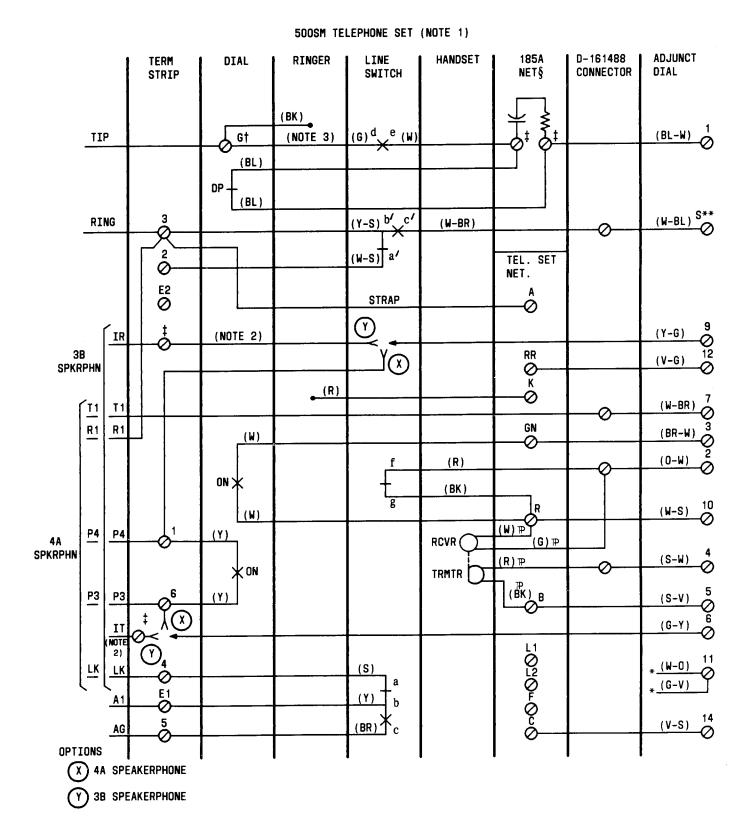
Fig. 14—1035C3A (MD) or 1035AF3A Dial, Connections to 500SM Telephone Set (Sheet 1 of 2)
