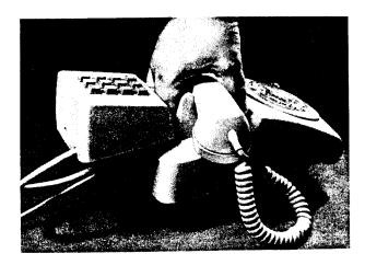
Fig. 5—1035C3A (MD) or 1035AF3A Dial Mounted on 500-Type Telephone Set Using 109B Bracket
