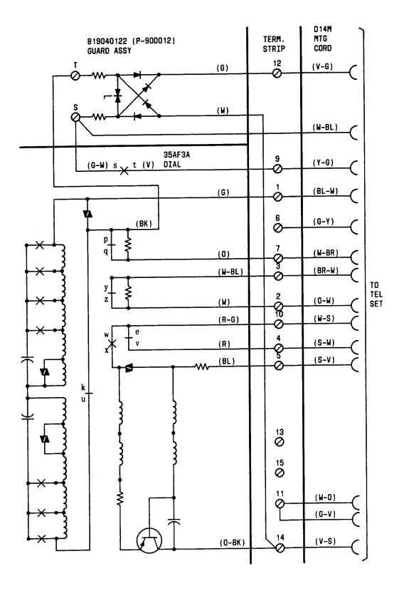
Fig. 11—♦1035AF3A Dial, Schematic
