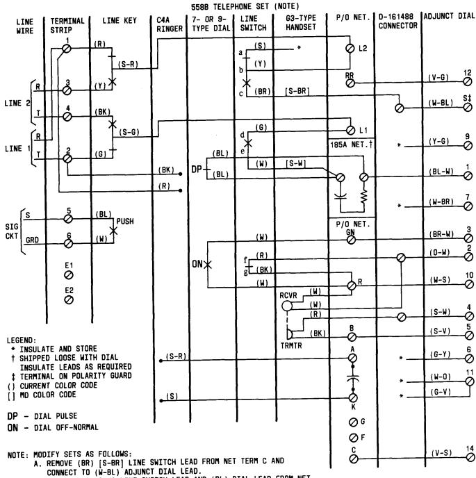
B. REMOVE (W) [S-W] LINE SWITCH LEAD AND (BL) DIAL LEAD FROM NET TERM F AND CONNECT BOTH TO ONE SIDE OF THE 185A NET.
