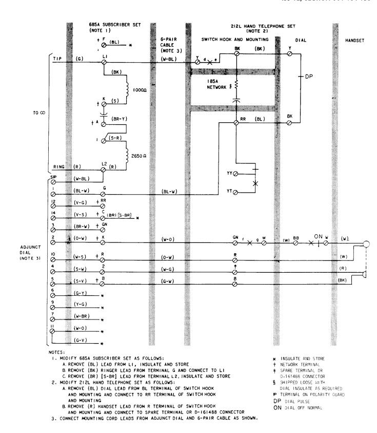
Fig. 12—1035C3A (MD) or 1035AF3A Dial, Connections to 212L Hand Telephone Set
