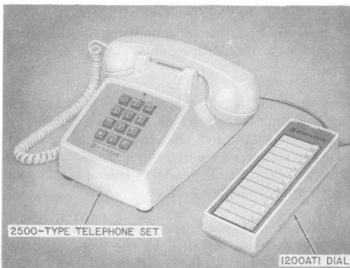
Fig. 1—Adjunct Dial and Associated Telephone Set
