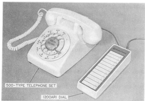
Fig. 1—Adjunct Dial and Associated Telephone Set
