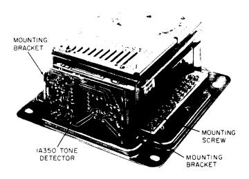
Fig. 3—1A350 Tone Detector, Installed
