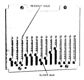
Fig. 2—43A Dial Coding Board
