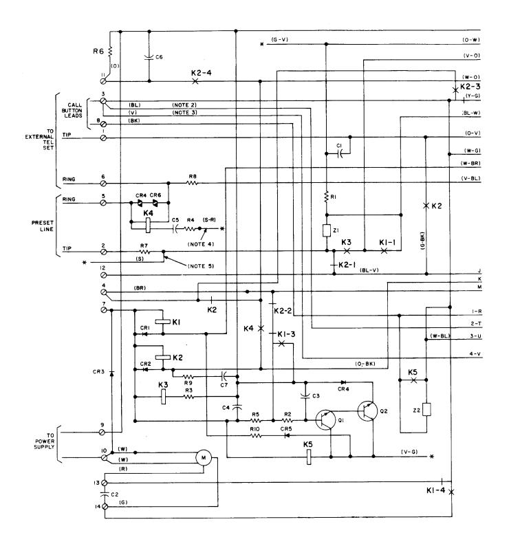
Fig. 11—43A Dial Connections, Factory Wired (Sheet 1 of 2)
