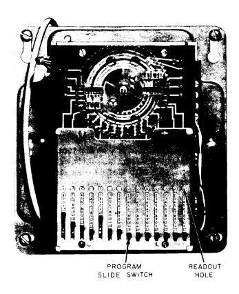
Fig. 1—53A Dial With Cover Removed
