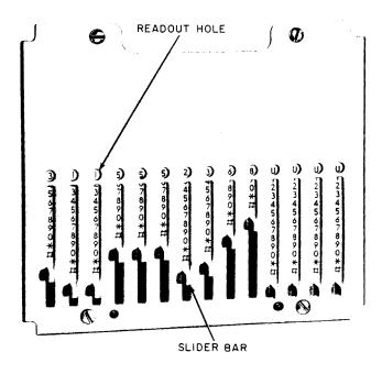
Fig. 2—53A Dial Coding Board
