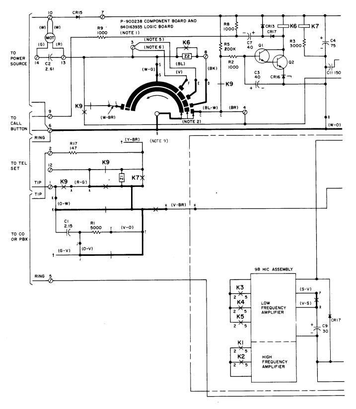
Fig. 11—♦53A Dial Connections, Factory Wired (Sheet 1 of 2) ♦
