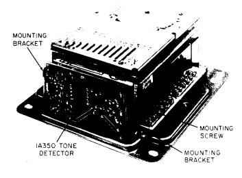
Fig. 3—1A350 Dial Tone Detector, Installed
