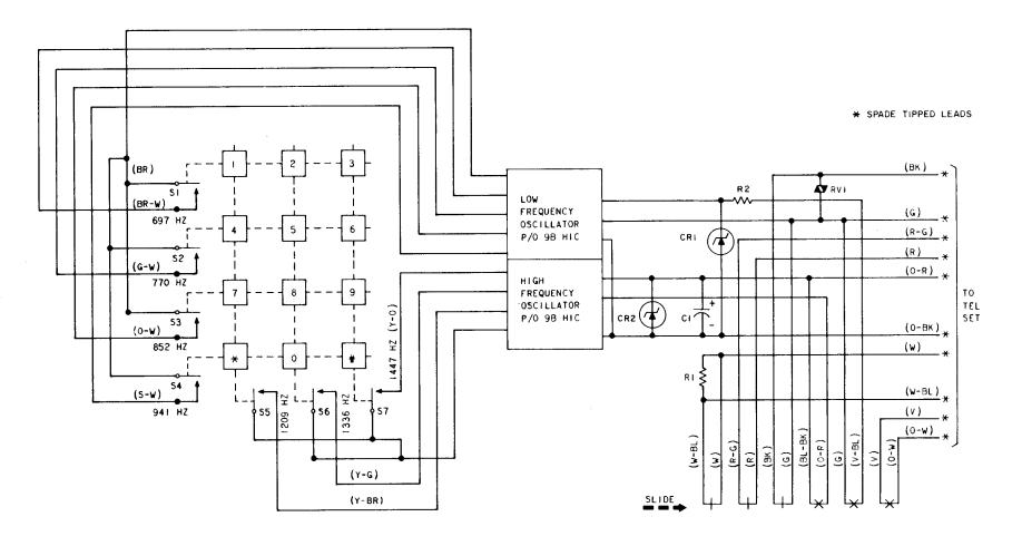
Fig. 2—70A Dial, Schematic
