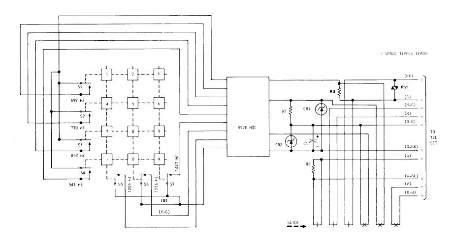
Fig. 3—♦70B Dial, Schematic
