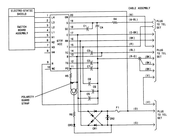
♦Fig. 15—Z72JG3B Dial, Schematic
