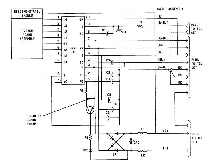
₱Fig. 16—Z72JG3BE Dial, Schematic¶
