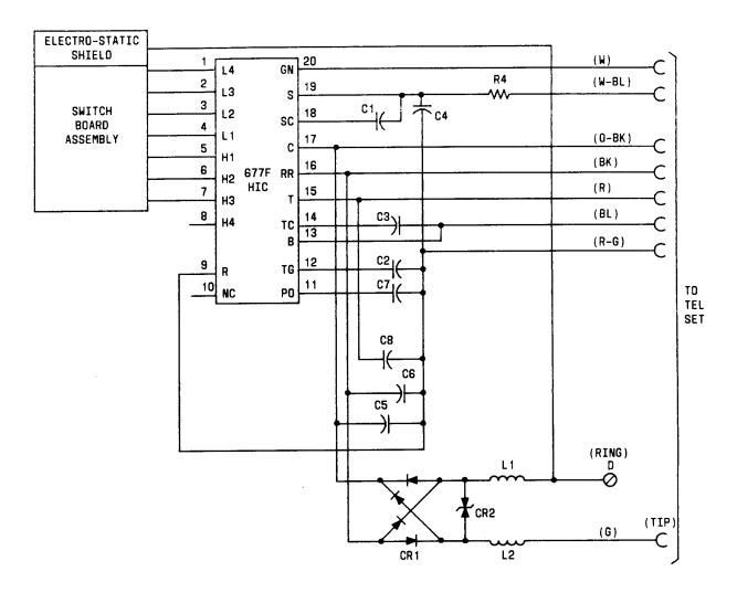
₱Fig. 12—Z72H3AE, Z72J3AE, or Z72K3AE Dial, Schematic¶
