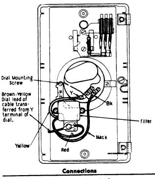
Terminal **Filter Lead** Transfer brown-yellow switchhook lead from Y of dial to filter bracket terminal. Connect yellow filter lead to Y of dial. Yellow Red To filter bracket terminal. Black To BK of dial.
